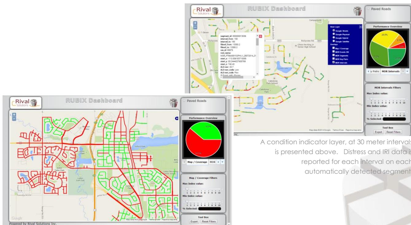
A condition indicator layer, at 30 meter intervals is presented above. Distress and IRI data is reported for each interval on each automatically detected segment.
